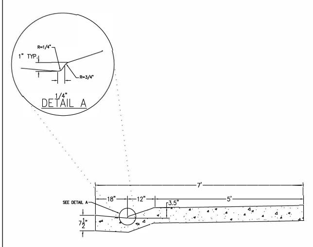
COMBINATION CURB, GUTTER, SIDEWALK
